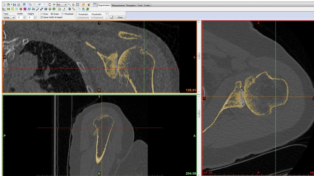
Figure F.5: In this case, connected pixels were deleted in order to separate the scapula from humerus.
